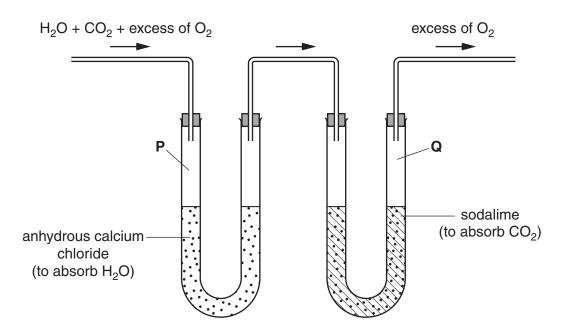
The increases in mass of the collecting vessels  ${\bf P}$  and  ${\bf Q}$  of the apparatus are  $M_{\rm P}$  and  $M_{\rm Q}$ , respectively.
