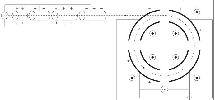
In the LINAC, the protons are accelerated from rest through 3 gaps each with an accelerating p.d. of  $36\,\mathrm{kV}$ .
