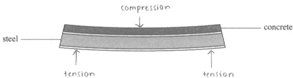
(a) (i) Label the diagram to show where the beam is under tension and under compression.
