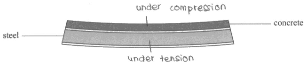
(a) (i) Label the diagram to show where the beam is under tension and under compression.
