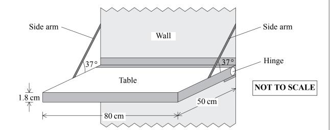
The table surface is 80 cm long, 50 cm deep and 1.8 cm thick. It is made from wood of density 0.70 g cm<sup>-3</sup>. Show that its weight is about 50 N.
