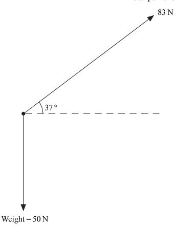
(i) Calculate the horizontal and vertical components of the 83 N force.
