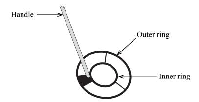
The outer ring contains the transmitter coil. Alternating current is passed through this coil. This creates a magnetic field which penetrates into the ground.
