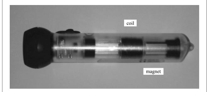
When the torch is shaken, the strong permanent magnet moves through the coil of copper wire, generating an electric current.
