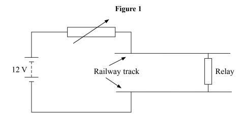
(a) The ratio of potential differences across the resistors in this circuit varies as the resistances change. What name is given to a circuit such as this which makes use of multiple resistors in this way?
