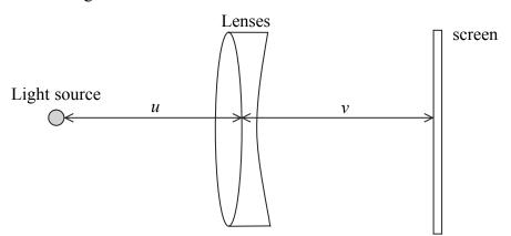
When the screen was moved back and forth, there was one point at which a clear image of the source could be seen on it.
