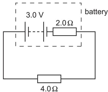
The battery is connected to a load of  $4.0\ \Omega$ .
