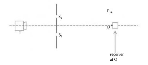
When the receiver is moved to P from O, which is equidistant from  $S_1$  and  $S_2$ , the signal received decreases from a maximum to a minimum. Which one of the following statements is a correct deduction from this observation?
