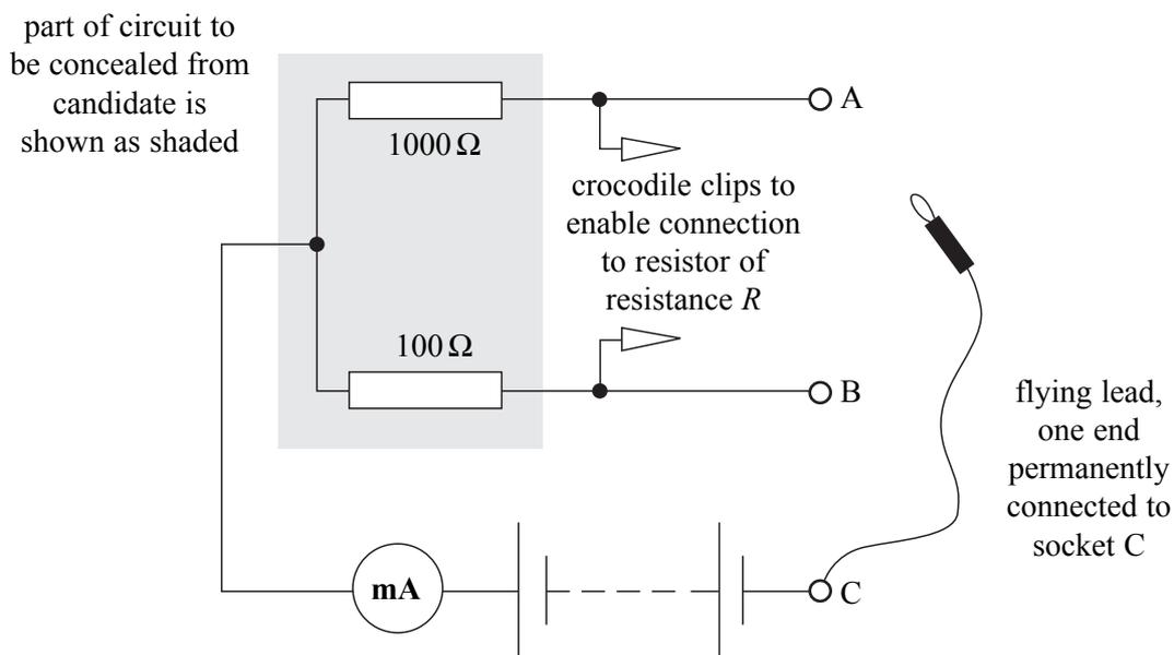
The crocodile clip connections should be arranged to provide easy insertion of the resistors, the resistances of which should be clearly marked for the candidates.
