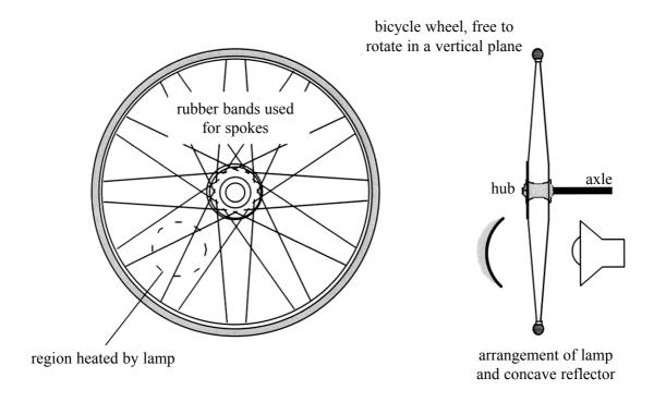
The spokes of a bicycle wheel have been replaced by rubber bands. Using a combination of a lamp and a concave reflector, heat is directed at part of the wheel. This makes the rubber contract and causes the position of the centre of mass of the wheel to move above the hub. As a result the wheel starts to turn and after a few seconds reaches a steady rate of rotation of about 1 rotation per second.
