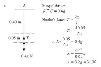
The modulus of elasticity is 31.4 N (3 s.f.)
