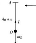
A particle attached to one end of an elastic string will oscillate about the equilibrium position. When solving problems about vertical oscillations, you often have to begin by finding the point of equilibrium. In this case, the oscillations later in the question have centre O.
