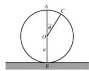
A particle is at the highest point A on the outer surface of a fixed smooth sphere of radius a and centre O. The lowest point B of the sphere is fixed to a horizontal plane. The particle is projected horizontally from A with speed u, where  $u < \sqrt{(ag)}$ . The particle leaves the sphere at the point C, where OC makes an angle  $\theta$  with the upward vertical, as shown in the diagram above.
