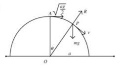
R is the reaction between the particle and the surface.
