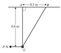
The figure shows a particle C of mass 2 kg suspended by two strings. The strings are fixed to two points A and B on a horizontal ceiling, where  $AB = 0.3 \,\mathrm{m}$ . The string AC is light and inextensible, with length 0.4 m, while the string BC is light and elastic with natural length 0.4 m and modulus of elasticity 32 N. A horizontal force of magnitude P N holds the system in equilibrium with AC vertical.
