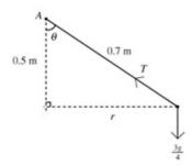
Let the tension in the string be T, and the angular speed be  $\omega$ . The angle between the string and the vertical is  $\theta$ , and the radius of the circle is r.
