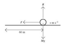
Let the mass of the car be M. Let F be the force due to friction between the car tyres and the road, and R the normal reaction between the car and the road.
