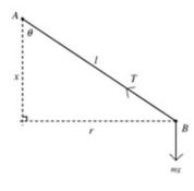
Let the tension in the string be T. The angle between the string and the vertical is  $\theta$ , and the radius of the circle is
