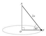
A particle P of mass m is attached to one end of a light inextensible string of length 2a. The other end of the string is fixed to a point A which is vertically above the point O on a smooth horizontal table. The particle P remains in contact with the surface of
