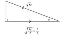
After leaving the hemisphere the horizontal component of the velocity remains constant. Direction is angle  $\alpha$  to the ground,
