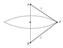
A particle P of mass m is attached to the ends of two light inextensible strings AP and BP each of length l. The ends A and B are attached to fixed points, with A vertically above B and AB = l, as shown in the diagram. The particle P moves in a horizontal circle with constant angular speed  $\omega$ . The centre of the circle is the mid-point of AB and both strings remain taut.
