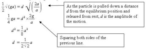
d As  $a > \frac{1}{2}a$ , the string will become slack during its motion. The subsequent motion of P will be partly under gravity, partly simple harmonic motion.
