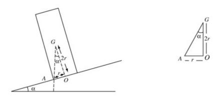
The diagram shows the limiting case when the point vertically below the centre of mass G is on the edge of the area of contact.
