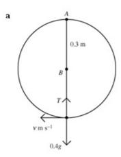
Let the speed of the particle at the lowest point be  $v \, \mathrm{m \ s^{-1}}$ , and the tension in the rod be  $T \, \mathrm{N}$ . At the lowest point the particle has fallen a distance 0.6 m, so the P.E. lost =  $0.4 \times \mathrm{g} \times 0.6$ ,
