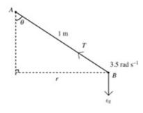
Let the tension in the string be T. The angle between the string and the vertical is  $\theta$ , and the radius of the circle is r.
