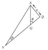
Let V be the vertex of the cone and O be the centre of its base. Let G be the position of its centre of mass.
