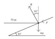
R is the normal reaction between the car and the track, F is force due to friction. At maximum speed F acts down the slope and is equal to  $\mu R = 0.4R$
