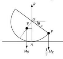
Draw a diagram showing O above the point of contact with the weight of P acting to one side and the weight of C balancing on the other side.
