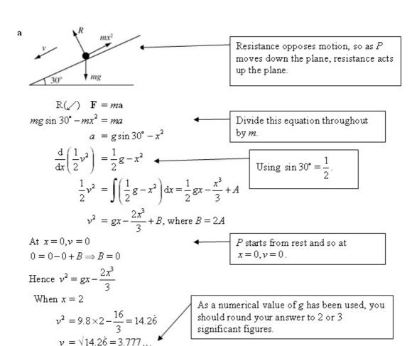
The speed of P when x = 2 is  $3.78 \,\mathrm{m \ s^{-1}}$  (3 s.f.)
