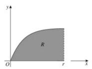
The diagram shows the region R bounded by the curve with equation  $y^2 = rx$ , where r is a positive constant, the x-axis and the line x = r. A uniform solid of revolution S is formed by rotating R through one complete revolution about the x-axis.
