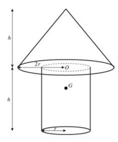
A model tree is made by joining a uniform solid cylinder to a uniform solid cone made of the same material. The centre O of the base of the cone is also the centre of one end of the cylinder, as shown in the diagram. The radius of the cylinder is r and the radius of the base of the cone is 2r. The height of the cone and the height of the cylinder are each h. The centre of mass of the model is at the point G.
