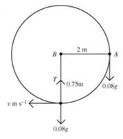
Let the speed of the particle at the lowest point be  $v \text{ m s}^{-1}$ , and the tension in the rod be T N.
