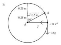
Let the speed of the particle where AB is horizontal be  $v \, \mathrm{m \ s^{-1}}$ , and the tension in the rod be  $T \, \mathrm{N}$ . At the point where AB is horizontal, the particle has fallen a distance  $0.5 \cos 60^{\circ} = 0.25 \, \mathrm{m}$ , so the P.E. lost  $= 0.6 \times g \times 0.25$ ,
