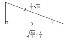
After leaving the hemisphere the horizontal component of the velocity remains constant.
