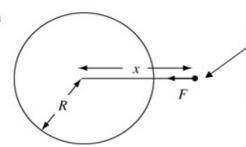
The gravitational force is directed towards the centre of the Earth and so is in the direction of x decreasing.
