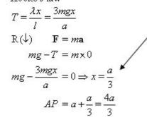
It is usually easier, when using Hooke's law, to work in terms of the extension of the string than to work with the total length of the string. Here, first find the extension when the acceleration is zero and, then, find the total length by adding the extension to the natural length.
