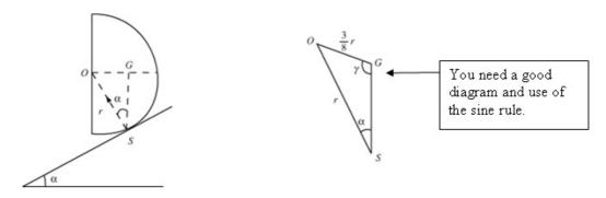
The diagram shows the equilibrium position with the centre of mass G vertically above the point of contact with the plane S. O is the centre of the plane face of the hemisphere.
