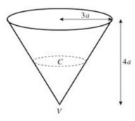
A hollow cone, of base radius 3a and height 4a, is fixed with its axis vertical and vertex V downwards, as shown in the diagram. A particle moves in a horizontal circle with centre C, on the smooth inner surface of the cone with constant angular speed
