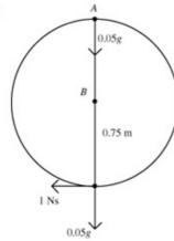
Impulse = change in momentum, so if the initial speed of the bead is  $u \text{ m s}^{-1}$  then
