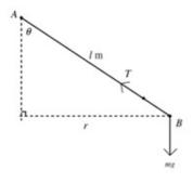
Let the tension in the string be T. The angle between the string and the vertical is  $\theta$ , and the radius of the circle is
