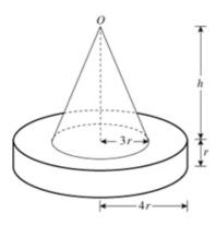
An experimental plastic traffic bollard B is made by joining a uniform solid cylinder to a uniform solid right circular cone of the same density. They are joined to form a symmetrical solid, in such a way that the centre of the plane face of the cone coincides with the centre of one of the plane faces of the cylinder, as shown in the diagram. The cylinder has radius 4r and height r. The cone has vertex O, base radius 3r and height h.
