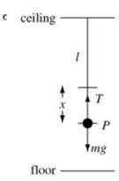
The maximum speed occurs when the acceleration is zero. Let the extension of the string at this point be x.
