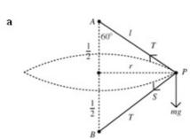
T is the tension in AP and S is the tension in BP. The triangle is equilateral (3 equal sides).
