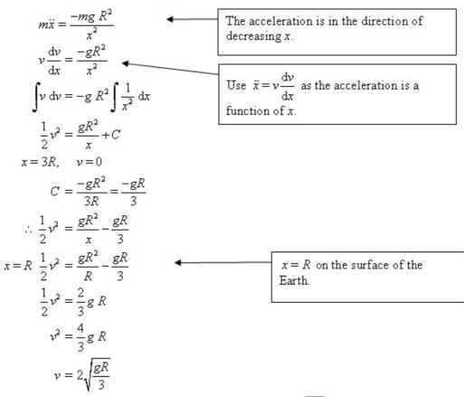
The particle hits the surface of the Earth with speed  $2\sqrt{\frac{gR}{3}}$
