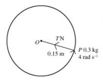
Suppose that the tension in the string is T. Using  $F = m\alpha$  $T = 0.3 \times 0.15 \times 4^2 = 0.72 \text{ N}$
