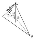
The diagram shows the equilibrium position with the centre of mass G, vertically below the point of suspension S.
