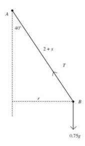
T is the tension in AB. AB is an elastic string, if the extension in the string is x then  $T = \frac{\lambda x}{l} = \frac{30x}{2}$
