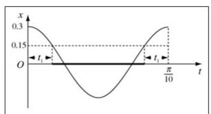
When the length of the spring is less than 0.75 m, the extension of the spring, x m, is less than 0.15 m. This sketch shows you that if the first time where the extension is 0.15 m is  $t_1$  s, the length of time for which the extension is
