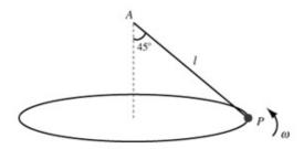
A particle P of mass m is attached to one end of a light string of length l. The other end of the string is attached to a fixed point A. The particle moves in a horizontal circle with constant angular speed  $\omega$  and with the string inclined at an angle of 45° to the vertical, as shown in the diagram.
