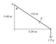
Let the tension in the string be T, and the angular speed be  $\omega$ . The angle between the string and the vertical is  $\theta$ . Since the triangle is right angled, the third side will have length 0.48 m (3, 4, 5 triangle).
