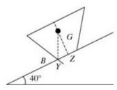
This time Y is vertically below G. Z is the centre of the circular face and B is the point about which toppling would occur.
