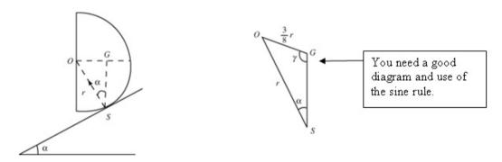
The diagram shows the equilibrium position with the centre of mass G vertically above the point of contact with the plane S. O is the centre of the plane face of the hemisphere.
