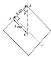
The diagram shows the equilibrium position with the centre of mass G below the point of suspension S.
