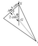
The diagram shows the equilibrium position with the centre of mass G, vertically below the point of suspension S.
