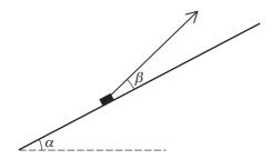
A small block of weight 5.1 N rests on a smooth plane inclined at an angle  $\alpha$  to the horizontal, where  $\sin \alpha = \frac{8}{17}$ . The block is held in equilibrium by means of a light inextensible string. The string makes an angle  $\beta$  above the line of greatest slope on which the block rests, where  $\sin \beta = \frac{7}{25}$  (see diagram). Find the tension in the string.
