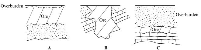
The ratio of the thickness of the overburden to the thickness of the deposit is known as the overburden ratio. An overburden ratio of 4:1 is close to the economic limit for low-value ores.
