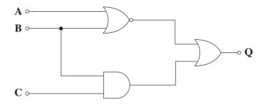
(i) In the space below, draw the same logic system, but with the logic gates replaced by their NAND gate equivalents.
