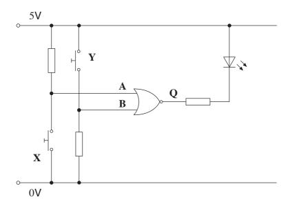
The table below shows the four possible logic states of switches  $\mathbf{X}$  and  $\mathbf{Y}$ . Complete the table by adding:
