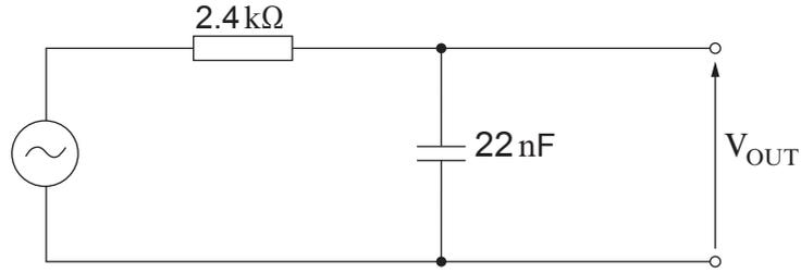
(a) What is the name of this type of passive RC filter? ..... [1]
