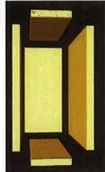
I decided to change how the box would be made, as it is now supporting a lot of weight. Thick side panels would be used as these will take the main strain from the above design. The back piece is also very thick so that the aluminium bars at the back will be held in place securely, and so that there is no chance of cracking.
