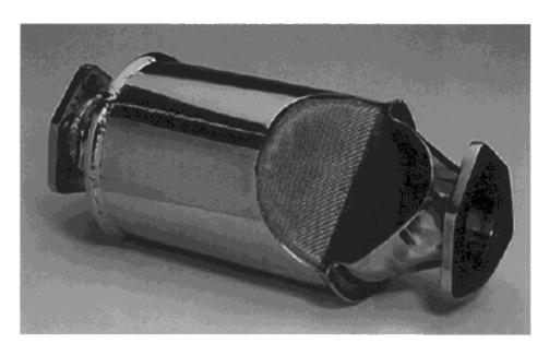
Explain why the honeycomb structure is used in a car exhaust system.
