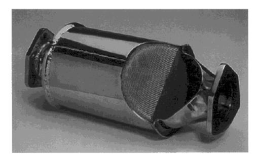
Explain why the honeycomb structure is used in a car exhaust system.
