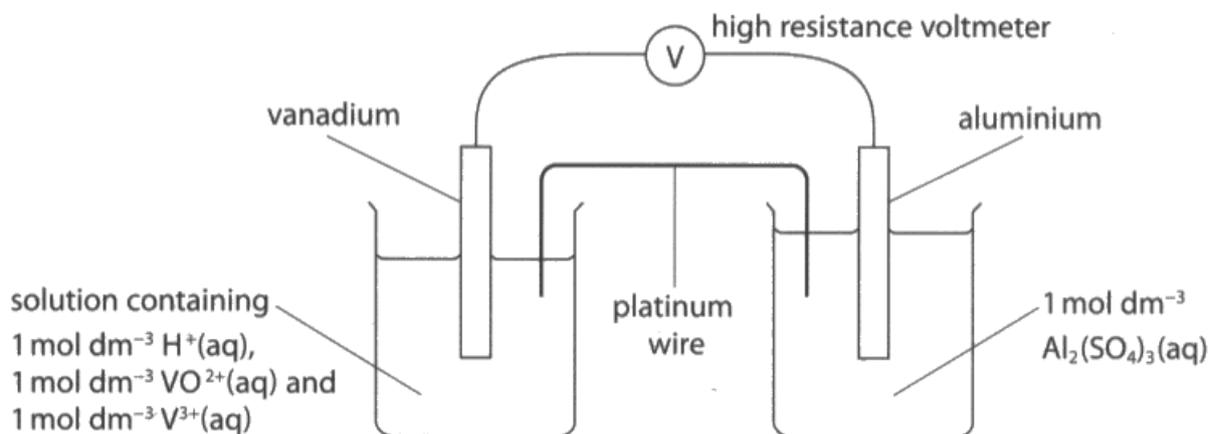
(e) Identify **three** mistakes in the way the cell has been set up and state what modifications should be made to correct them. Write your answers in the table below.
