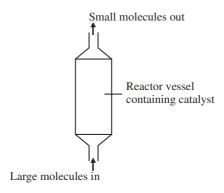
(i) Cracking involves a thermal decomposition reaction.
