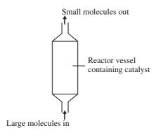
(i) Cracking involves a thermal decomposition reaction.
